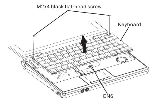
Figure 4-6 Removing the keyboard cover and keyboard
